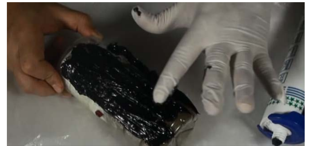
II. Spread the silicone uniformly all over the surface. The thickness of the silicone should be about half a centimetre.
