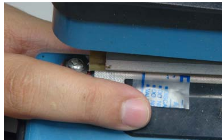
V. Seal three sides of the rectangle to make a small bag.
