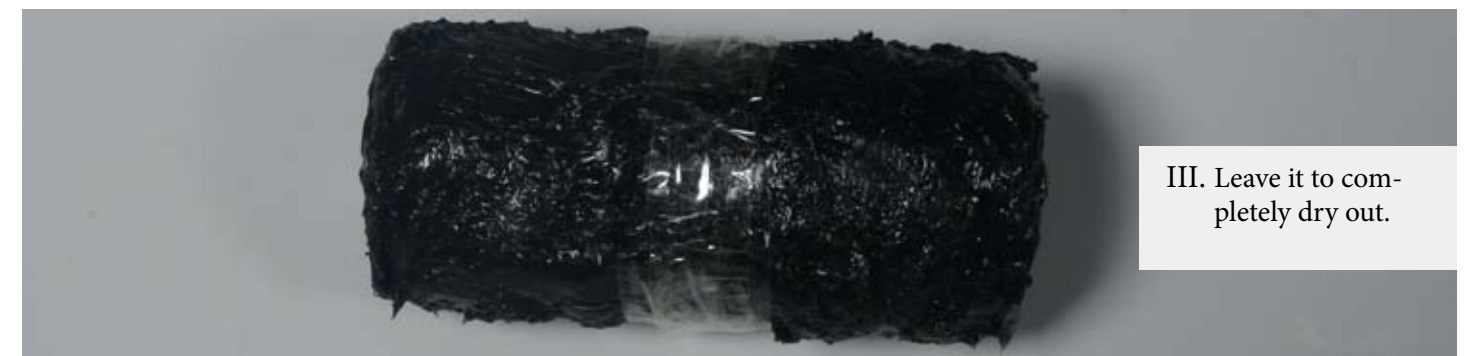
II. Spread the silicone uniformly all over the surface. The thickness of the silicone should be about half a centimetre.
