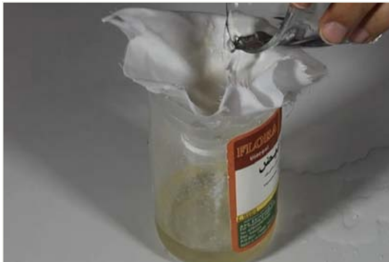
VII. Wash the white solid with water repeatedly for more than 20 TIMES to get rid of the acid that remains in the solid.
