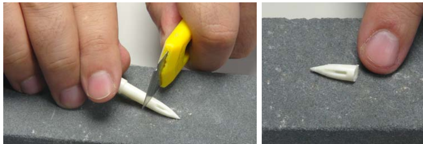
VIII. Cut the tip of a plastic drip needle.
