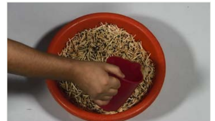
II. Pour 5 litres of hot water on the matchsticks. Stir well. All of the chlorate will dissolve in the water.
