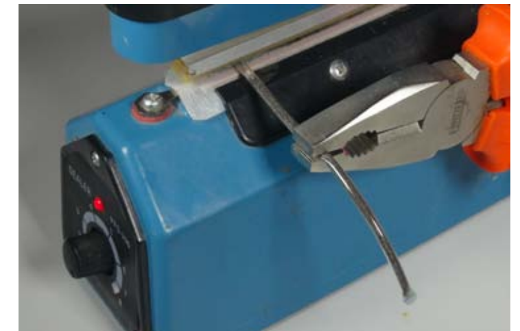
VI. Seal the end with a heat sealer. You should hold the pipe/fuse with a pair of pliers for safety purpose.
