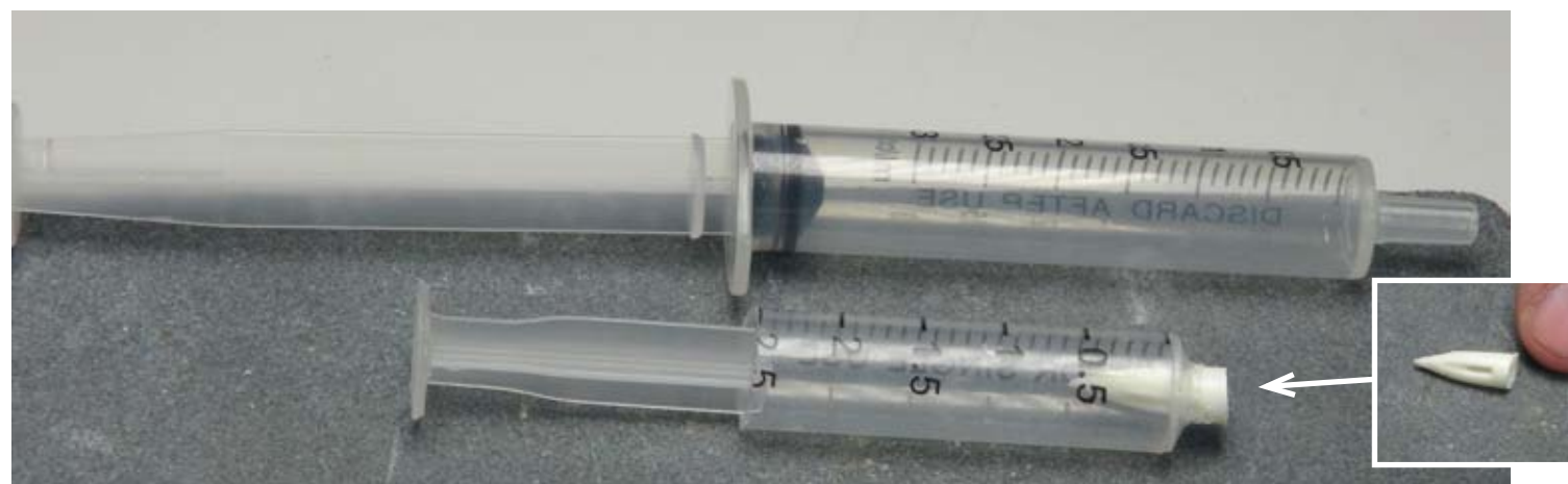
IX. Take a 3 ml syringe and cut it as illustrated above. Then make a hole in the bottom of the syringe and insert the plastic drip needle.
