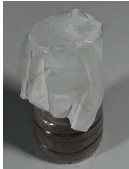
V. Place a tissue paper on the open side of the bottle, fasten it with a scotch tape.
