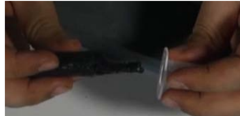
V. Cut the top of a 10 ml syringe and insert the explosion starter so that it helps in pushing the plunger.
