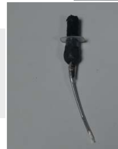
VI. Join one burning fuse with the percussion cap using a scotch tape. Fasten the lower part of the explosion starter with epoxy.
