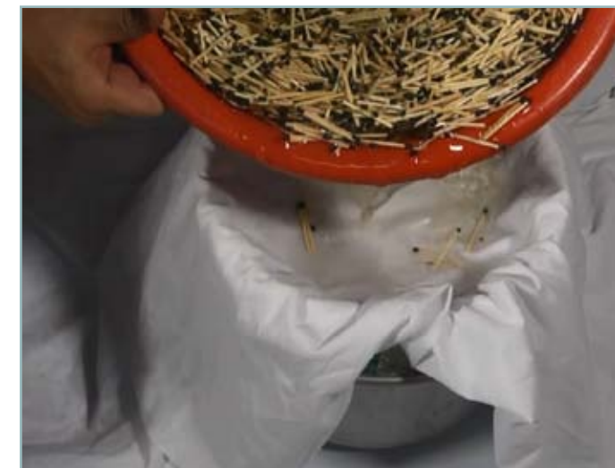
III. We need to separate the water from the sticks. Place a piece of cloth on a container to act as a filter and pour the mixture on the cloth.
