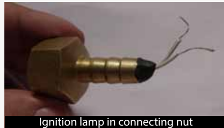
Ignition lamp in connecting nut
