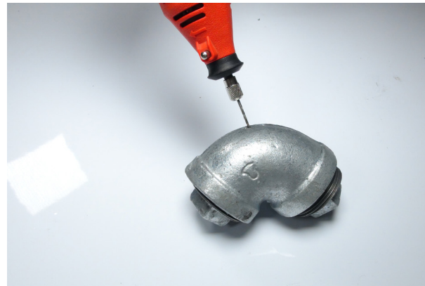
2. Drill a small hole as shown.
